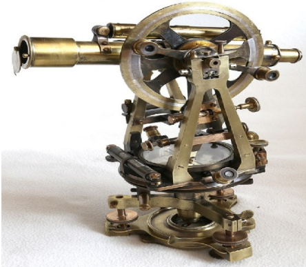
Fig 2.31- A theodolite of 1851
