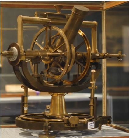
Fig 2.31- A theodolite of 1851
